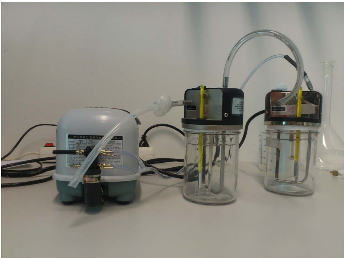
Figure 1: Experimental setup for the breathalyzer study with the membrane pump to the left, and the two simulators operated in series on the right. The calibration gas is provided through the silicon tubing. Simulators are not filled.
